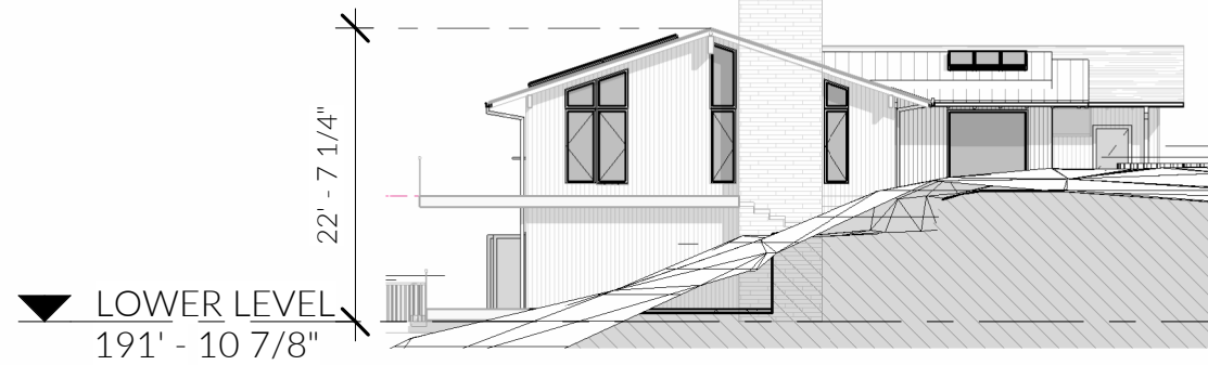
7 SIDE YARD CALCULATION FACADE HEIGHT DIAGRAM 1/16" = 1'-0"
