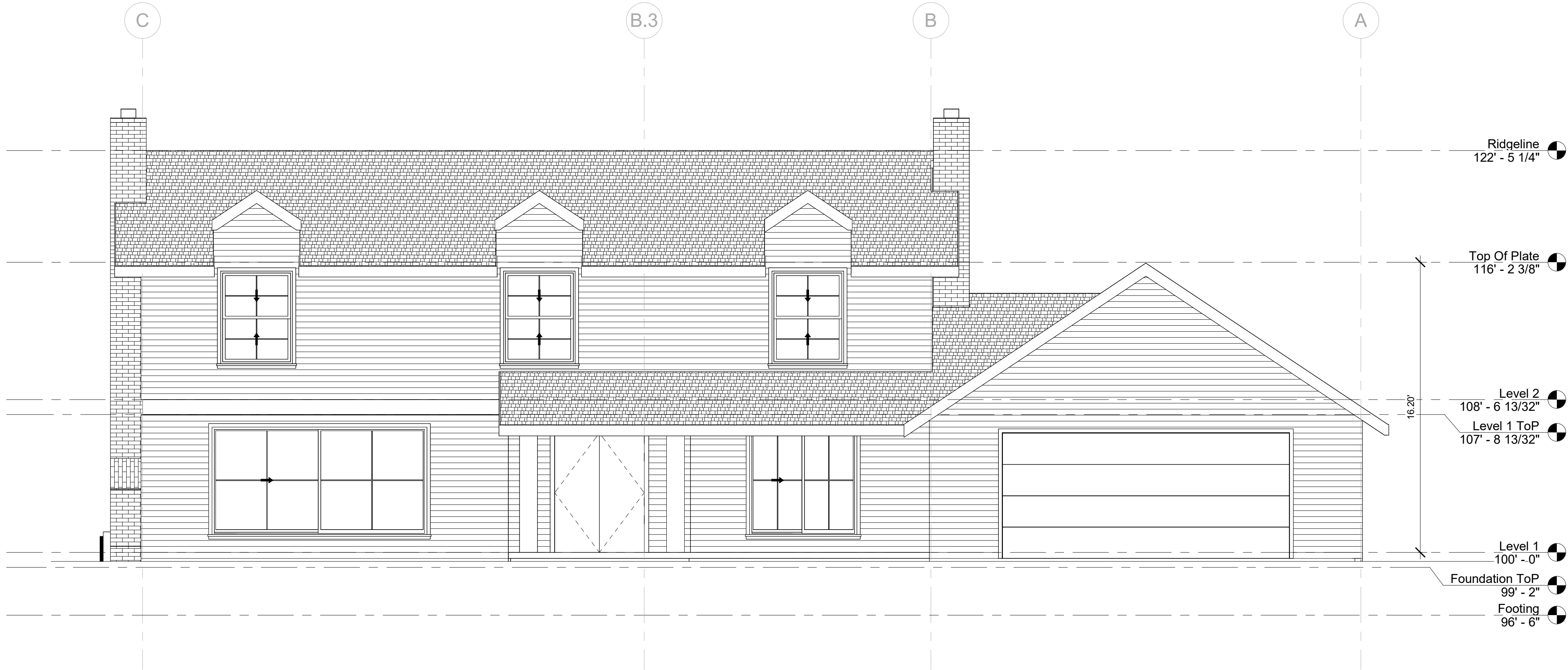
2 SOUTH (FRONT) ELEVATION SCALE: 1/4" = 1'-0"
