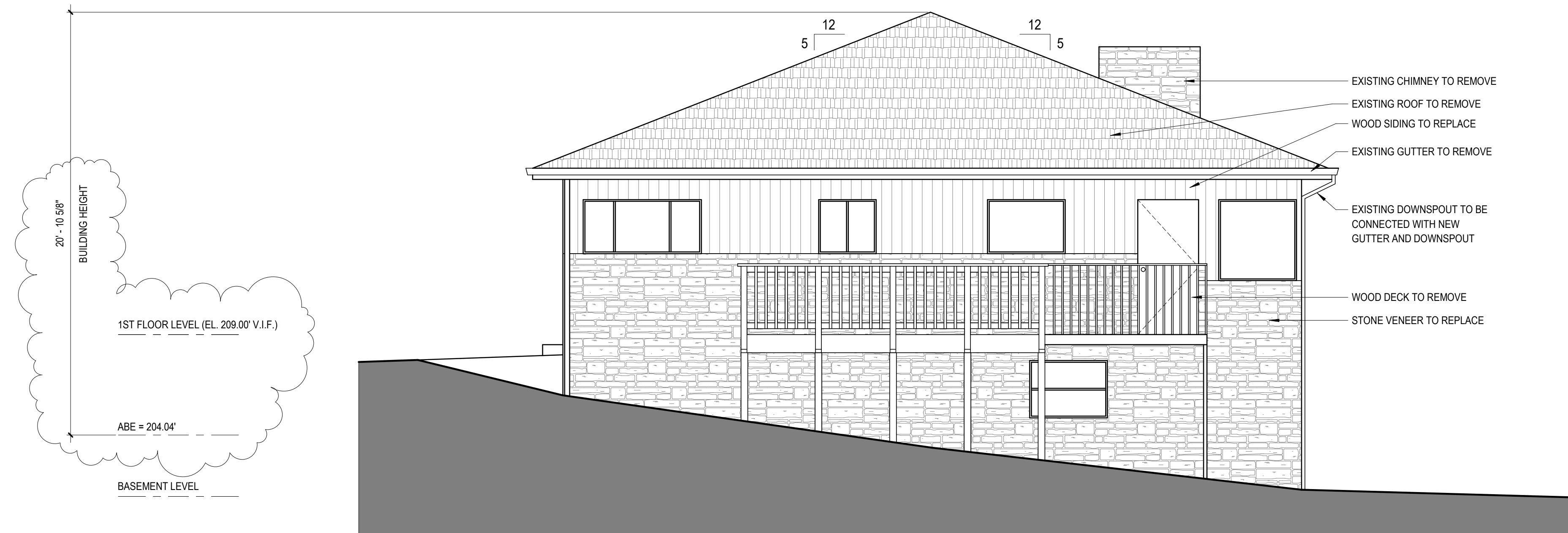
1 BUILDING ELEVATION EAST - EXISTING 1/4" = 1'-0"
