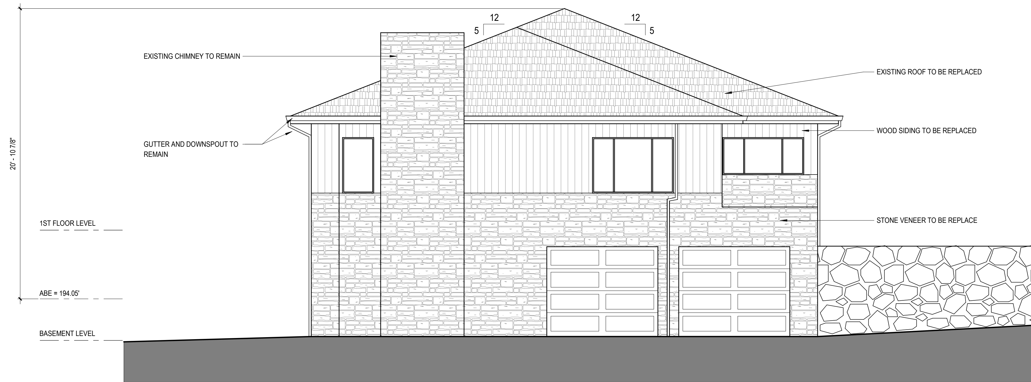
1 BUILDING ELEVATION WEST - EXISTING 1/4" = 1'-0"
